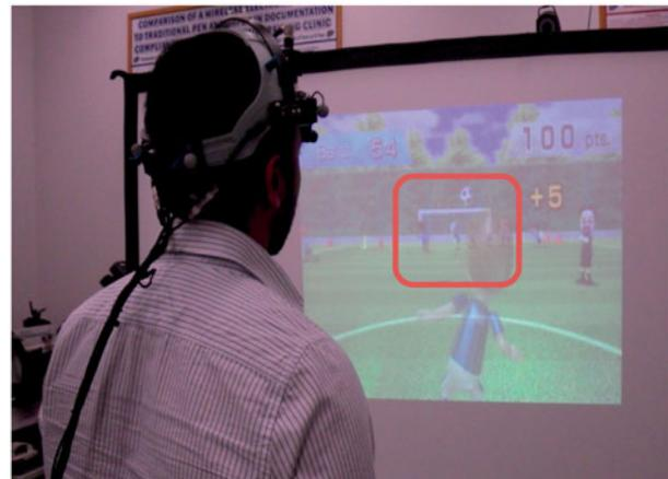
Figure 2. Experimental set-up: the participant wore a head mounted eye tracking system. In front, the Wii Soccer game was displayed. The participant stood on the Wii Balance Board to direct the Mii (avatar) to head soccer balls while dodging distracter items. The defined centre of screen for gaze analysis is indicated by the square on the screen.
