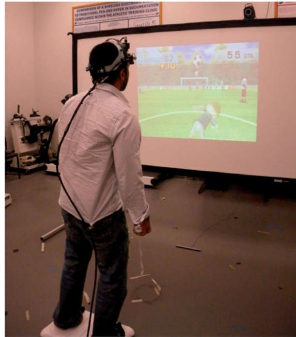
Figure 1. Full body experimental set-up: both feet are centred on the force plate sensors of the WiiFit platform.
